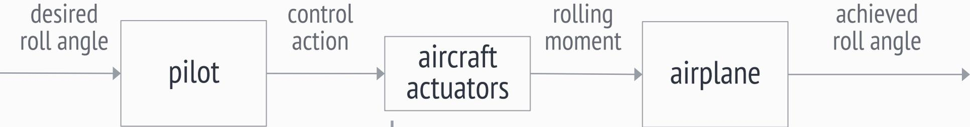
***actuators** are the things that move, e.g. moving surfaces on the wing*
